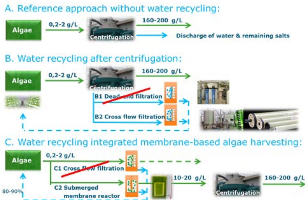
Figure 8. Schematic overview of different approaches for harvesting and medium recycling.
