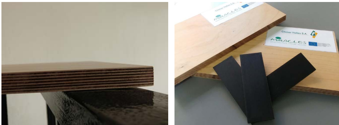
Figure 22. Plywood panels and coating material produced using algae based resins
